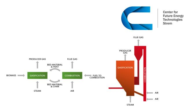
The synthesis gas produced during the gasification in the DFB gasifier contains little nitrogen and has an appropriate H2/CO ratio. The gas with this H2/CO ratio and the lack of nitrogen has a much higher heating value than the product gases of other gasifiers and is also very well suited for chemical synthesis. Due to the high calorific value, the gas is particularly well suited for use in motors for generating electricity.
