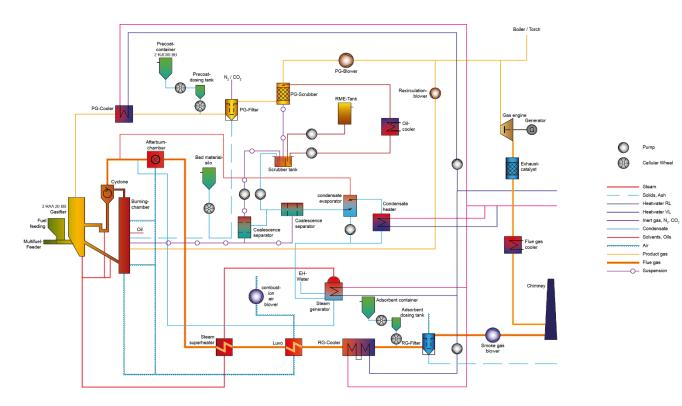
The main components of DFB gasification are shown in the following scheme:
